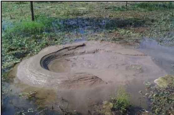
Photograph IV-9. Sand Cone on Flowing Boil
