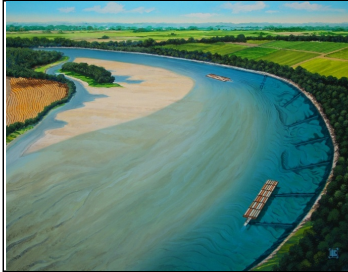
Figure IV-9. Illustration of Bendway Weirs
