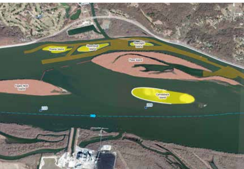
Canvasback Island, eight miles from Alton, was created by dredged material to mimic the original sandbar islands of the Mississippi and provide habitat for wild life like the Interior Least Tern. BELOW, FROM LEFT: The islands, situated on this map, were designed to last at least 50 years and, when above water, to provide bird nesting areas and also benefits to fish, wildlife and boating access. Terns responded quickly, nesting on the new island for three consecutive years. Partners banded the baby terns to test the islands' nesting success.
