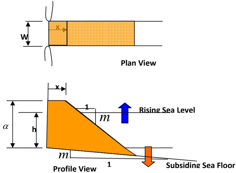
Figure 7. Uniform width model. Sloping sea floor.
