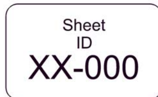
Figure 3-6. Sheet identification block
