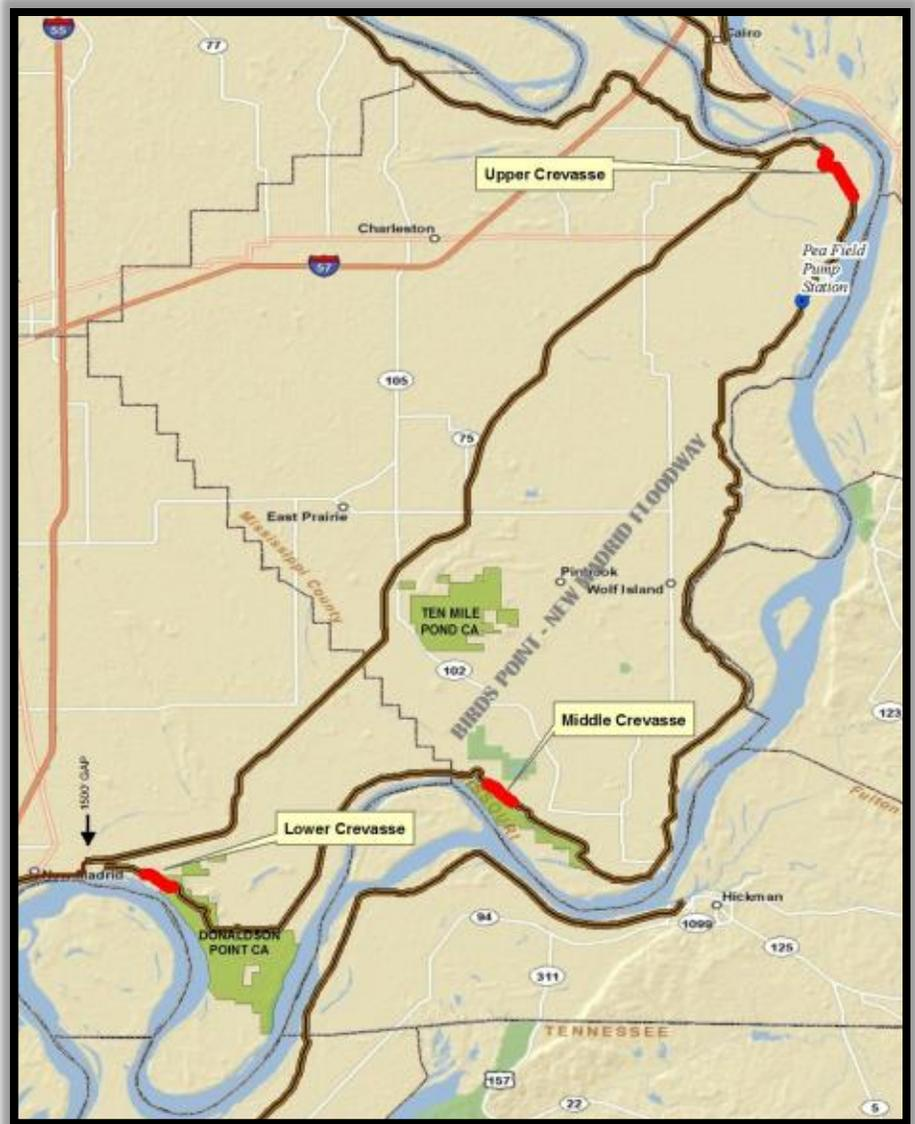
This site is used to both introduce floodwaters upon floodway activation and to drain the floodway after the flood crest passes. The 5-mile-long lower crevasse consists of approximately 3.5 miles of lowered fuseplug levee for overtopping and 1.5 miles of raised
