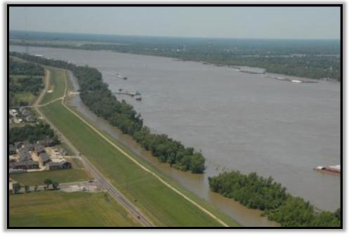
purchasing the land within the floodway; constructing permanent auxiliary channels in the floodway to confine floodwaters diverted into the area, rather than allow them to overflow the entire floodway; realigning and setting back the frontline levee at five locations
