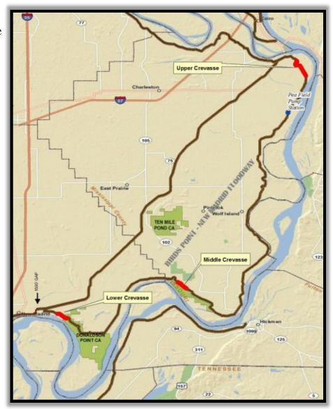
This site is used to both introduce floodwaters upon floodway activation and to drain the floodway after the flood crest passes. The 5-mile-long lower crevasse consists of approximately 3.5 miles of lowered fuseplug levee for overtopping and 1.5 miles of raised sections of levee that that are imbedded with pipes. The lower crevasse site also acts as an inflow and outflow location.
