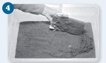
Next, press damp sand into the bottom of a shallow rectangle box. As in Step 2, move the ice block gravel-and-rock side down along the surface of the sand while pressing down lightly.
