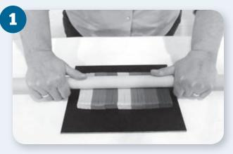
Using a rolling pin or large dowel, flatten the modeling clay into a rectangle approximately  $20 \times 10 \times 1$  cm.
