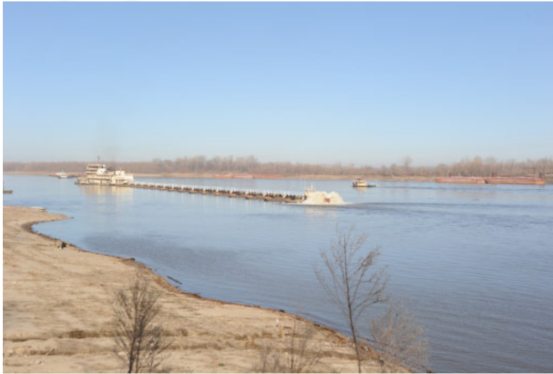
The Dredge Potter, one of the Corps' dustpan dredges, removes sediment from the mainstem Mississippi River channel to keep commercial navigation flowing during extreme low-water conditions between St. Louis, Mo., and Cairo, Ill. (Photo by the St. Louis District.)
